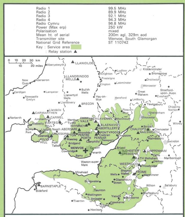
The service area is where the average field strength is not less than 54 dB (relative to  $1\mu V/m$ ) at a height of 10m. The service areas of the relays are not shown but technical details are listed overleaf.
